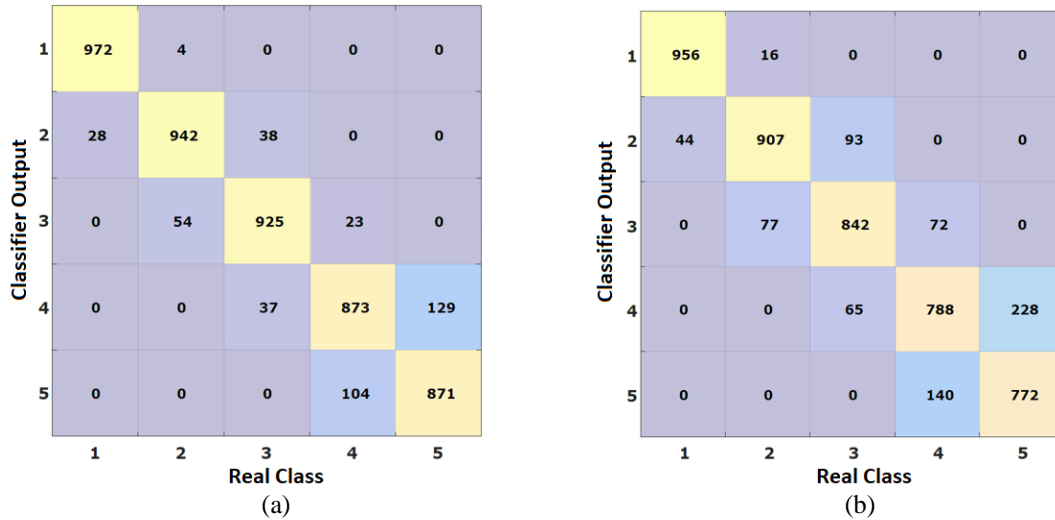
Figure 3: Confusion matrices for the Bayesian classifier using \varepsilon_1 , \varepsilon_2 and \varepsilon_3 with M = 128 (a) and M = 64 (b).
